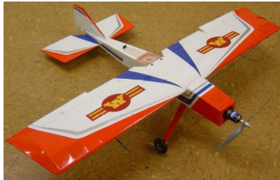
Fig. 2 The mini-UAV (Ultra Stick 25E RC plane)
